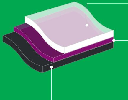
**Facestock:** 50 $\mu$  clear scratch resistant topcoated polyester offers excellent optical clarity and dimensional stability combined with good solvent, humidity, elevated temperature and UV resistance. Designed to be UV digital printed. The topcoating ensures excellent ink-adhesion combined with superior scratch resistance of non-printed areas.
